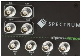
Standard BNC connectors are used for all analog input or output signals and all auxiliary signals like clock and trigger. No special adapter cables are needed and the connection is secure even when used in a moving environment.
