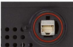
The GBit Ethernet connection can be used with standard COTS Ethernet cabling. The integration into a standard LAN allows to connect the digitizerNETBOX/generatorNETBOX either directly to a desktop PC or Laptop or it is possible to place the instrument somewhere in the
