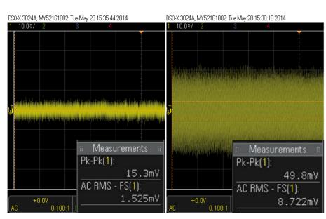
PS48402 output noise (20Hz-1MHz BW, 24V, 82Ω load)
