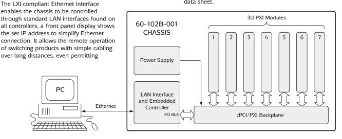
Plugging Pickering Interfaces PXI modules into the 60-102B LXI Modular Switching Chassis provides an LXI compliant switching platform. A simple Ethernet lead is the only physical control connection required.
