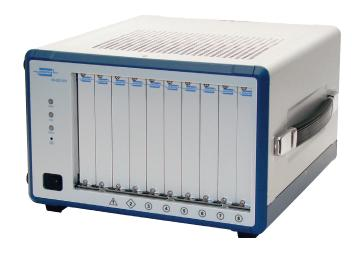
Two 60cfm fans insure maximum PXI module cooling and an efficient direct convection design allows the chassis to operate over an extended ambient temperature range of  $0^{\circ}$ C to  $+55^{\circ}$ C.
