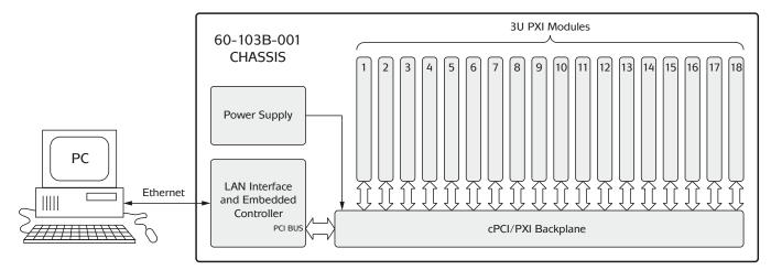
Plugging Pickering Interfaces PXI modules into the 60-103B LXI Modular Switching Chassis provides an LXI compliant switching platform. A simple Ethernet lead is the only physical control connection required.
