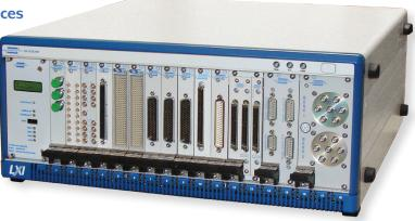
The 60-103B is fully compliant with the LXI Standard 1.4 and supports Pickering Interfaces 3U PXI switching and simulation modules. Each module is supported as though it is an LXI compliant device, complete with a driverless soft front panel that provides control of the module functions. The 60-103B supports up to 18 off 3U modules and is equivalent to a 19 slot PXI chassis.
