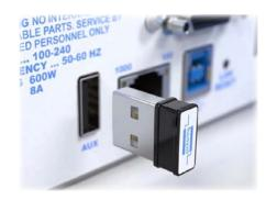
The 60-106 LXI/USB chassis can be controlled via cable using the Ethernet or USB 3 interface. Alternatively, it can be controlled wirelessly using the optional WiFi dongle.
